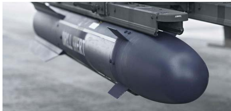
▲ MISSILE Up to 16 Hellfire guided missiles can be carried by the aircraft (a training round is shown above). These anti-armour weapons have a range of 8km (five miles).
